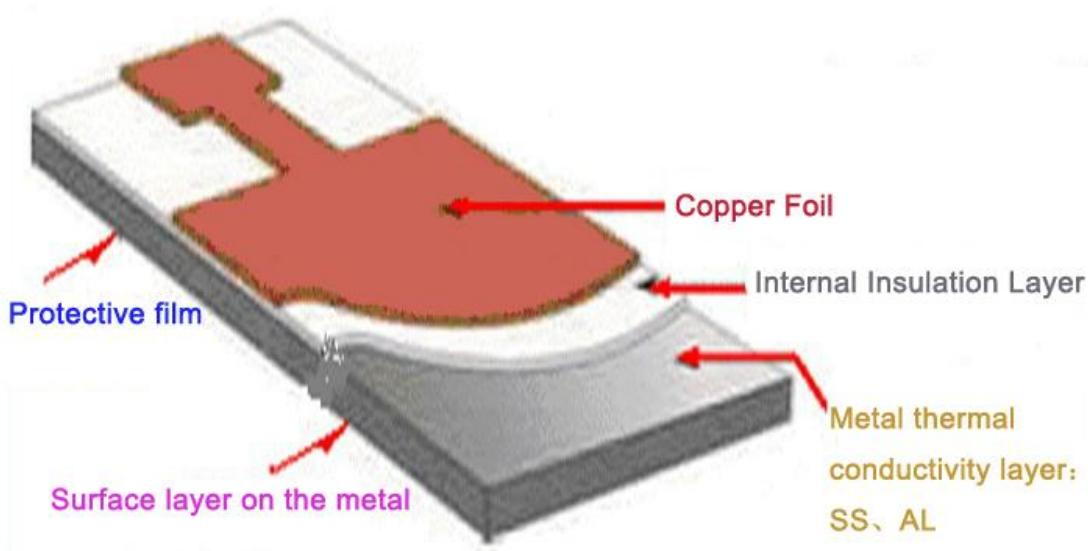
The above is the typical structure presentation of Al Copper Clad Laminates, Our company had successfully study out the thermal conductive materials with the low thermal resistance and high thermal conductivity through the research of resin formulation.
